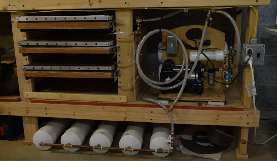
Building guitars requires a mix of traditional woodworking machinery and specialized fixtures. Some of the tools here I made, such as the router table below, the disc sander at bottom left and the soundboard vacuum press system on the left. Evolving the process and inventing the machinery to implement it is one of the great pleasures of this endeavor.
